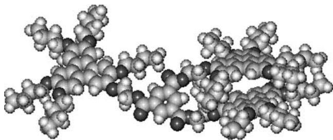
(c) IIIb , X=H, R=C 4 H 9 [9], swallow-tail conformation E = 143.2 kcal/ mol; MP : M_m = 1.24 , M_r = 0.62 , K_c = 1.97 , K_p = 1.63 , K = 5.02 , K_{ar} = 0.177 . Prediction with KM is (-).
